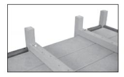
Place shelf in line with bottom rails on leg assembly and fasten with screws in the pilot holes. Be sure that screws go into the pilot holes in the leg assembly.
