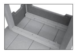
Place leg assemblies snugly against the tabletop crosspieces. Secure each leg assembly with four screws using the pilot holes.
