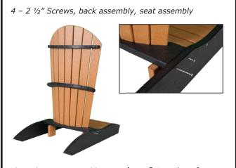
Place the seat assembly on a clean, flat work surface. Place the two spacer blocks close to the side rails of the seat assembly where the back attaches. Set the back on top of the space blocks. Push the back into the seat against the back seat slat. Fasten with the four 2  $\frac{1}{2}$ " screws using the pilot holes in the seat side rail.
