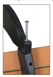
Place a washer on a 3" lag and fasten the back of the arm to the back of the chair. Be sure to place the lag in the pilot hole in the chair back.
