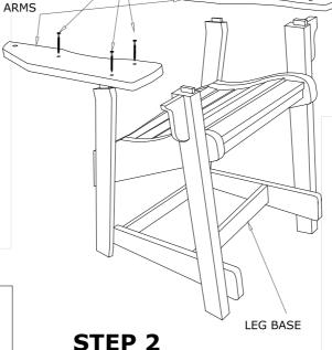
Attach arm rest and supports as shown.
